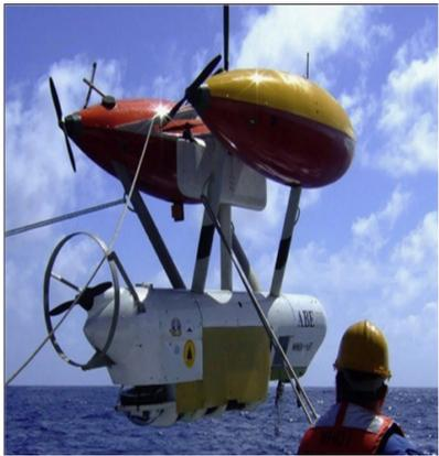
Figure 1. The autonomous benthic explorer (ABE) a free-swimming robot. In this image, ABE is about to be set loose to explore the bottom of the SW Indian Ocean from aboard the Chinese research ship Da Yang Yi Hao in 2007. Over the past five years, ABE has been used on multiple expeditions to find new hydrothermal vents in the deep ocean all over the world, from New Zealand to South Africa and Brazil to Ecuador. Click image for larger view and image credit.
