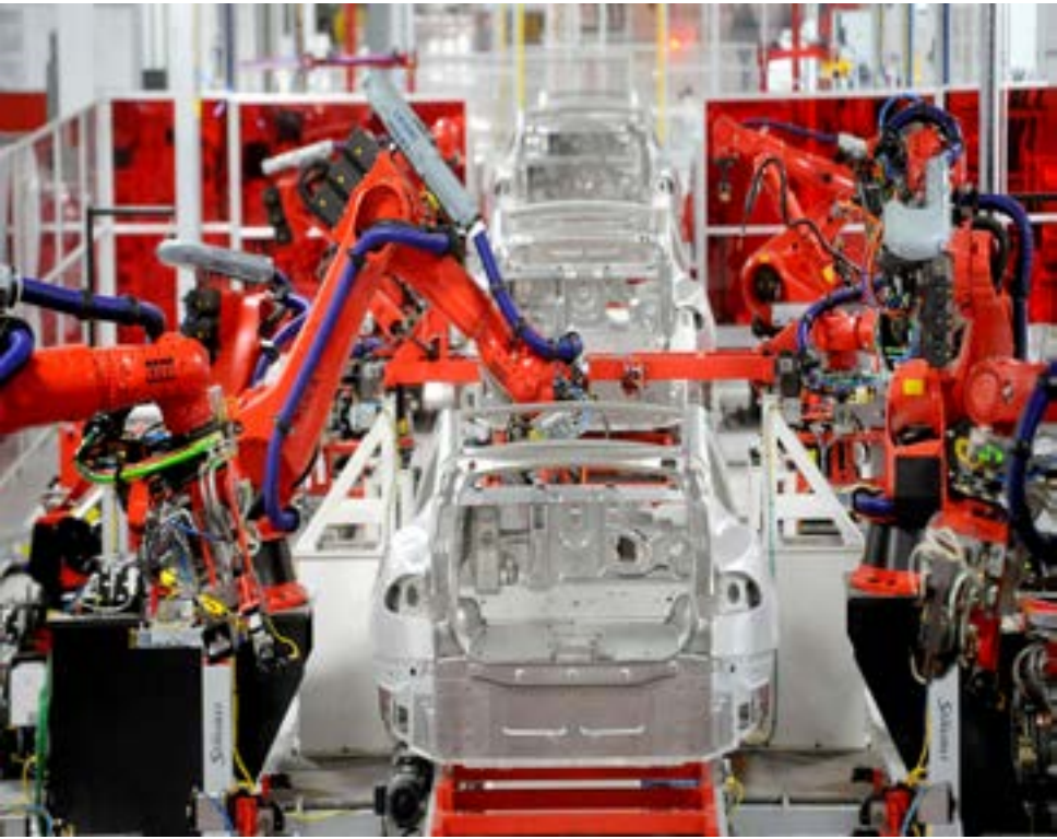
FILE PHOTO: Robotic arms assemble Tesla’s Model S sedans at the company’s factory in Fremont
